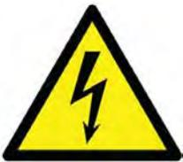
**DANGER - HAZARDOUS VOLTAGE** - placed on covers of the rectifiers and controllers, and inside of rectifiers (WILL CAUSE SEVERE SHOCK OR BURN).
