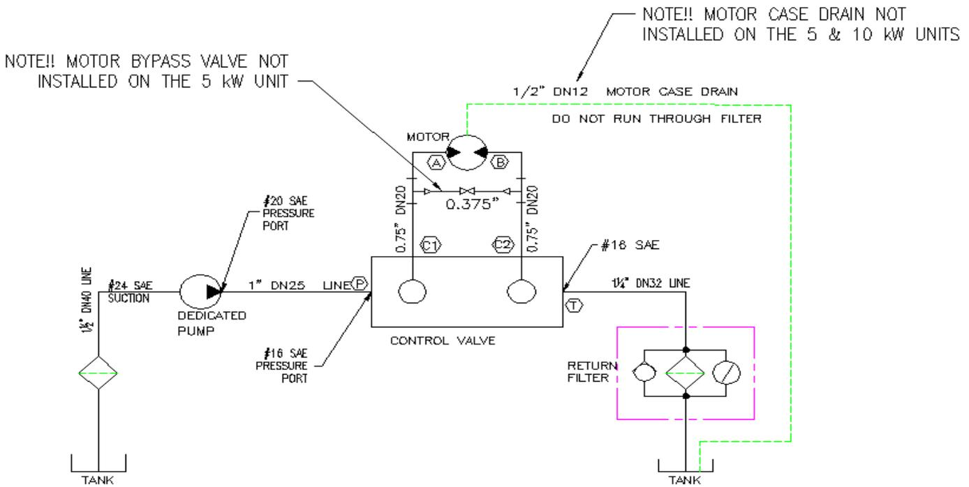
Fig. 1 Hydraulic Schematic
