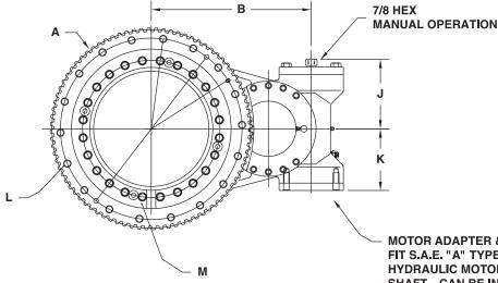
MOTOR ADAPTER & MOUNTING HOLES TO FIT S.A.E. "A" TYPE 2-BOLT STANDARD HYDRAULIC MOTOR WITH 1" KEYED SHAFT...CAN BE INSTALLED ON EITHER SIDE.
