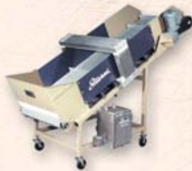
Inclined conveyor system with metal detector for monitoring a bulk bagged product, including bell alarm with belt stop reject system.
